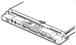
Figure 4-15 Detaching the Port Replicator
